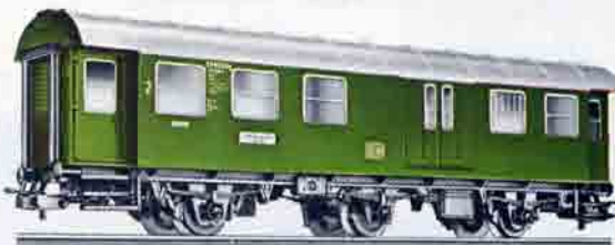
4080 PASSENGER CAR WITH BAGGAGE COMPARTMENT · Second class, six-wheeled coach · A model of the German Federal Railways type BD3yge · Dark green body with inset plastic window frames · Simulated rubber diaphragms on ends · Silver roof · Length 6" · Provision for fitting the 7074 lighting equipment (see page 56)
