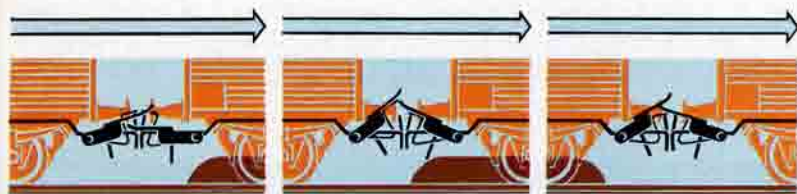
Raising the track ramp releases the couplers.
